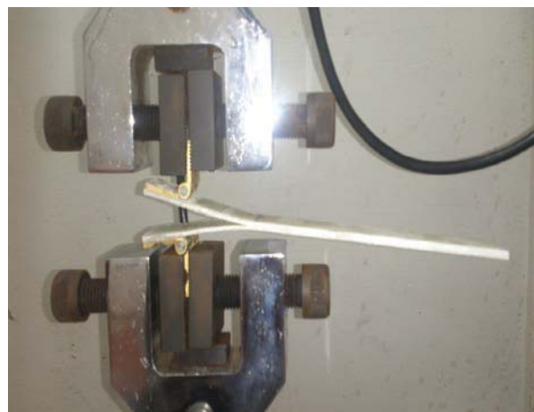
Fig. 3. Mode I fracture test.
