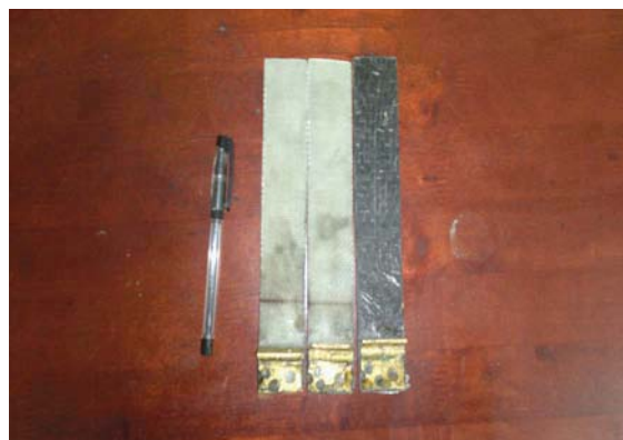
Fig. 4. Type I, II and III DCB specimen.
