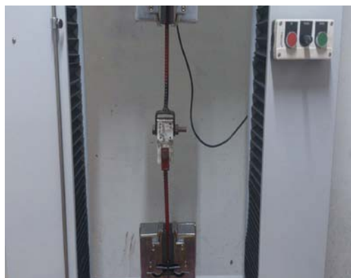
Fig. 2. Flat wise tension test.
